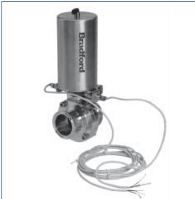
Bradford™ automated butterfly valve with vertical canister air-to-open spring-to-close actuator and proximity sensors. B5101S200CC-MI
