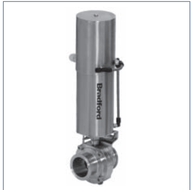
Bradford™ automated butterfly valve with vertical canister air-to-open spring-to-close actuator and control top, with 24VDC solenoid. B5101S200CC-ZB
