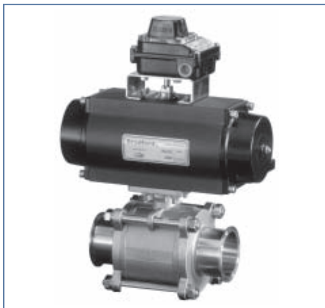
Bradford™ automated 2 1/2" 2-way encapsulated ball valve with spring return fail close actuator and NEMA 4/4X limit switch with two SPDT mechanical switches pictured. BV2CV-250CC-BFC .
