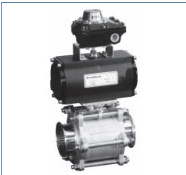
Bradford™ automated 3" encapsulated ball valve with direct mount double acting, (normally open), actuator and NEMA 7 (explosion proof with 2 mechanical switches) SPDT limit switch pictured. BV2CV-300CC-QAC .
