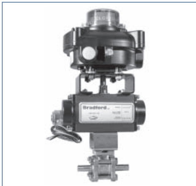
Bradford™ automated 1/2" encapsulated 2-way ball valve butt-welded ends, spring return actuator, and NEMA 7 (explosion proof) SPDT limit switch with two proximity switches and NEMA 7 NAMUR mount 24VDC voltage solenoid valve pictured. BV2CV-050BB-FPC .
